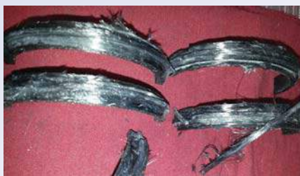
Polyetheretherketone bushings and wear rings from the fractionator pumps.
