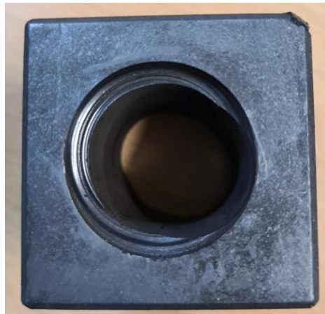
Wear of Original Plain Graphite Bearing
