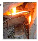
**Frequent breakdowns were occurring.** Due to the complex, precise motions involved and the extreme heat conditions, the trough positioning mechanism was experiencing frequent breakdowns. Alternative solutions allowed for precise positioning but failed under the harsh operating conditions.
