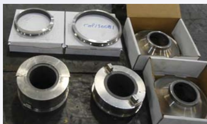
Replacing the old bushings and wear rings allowed the pumps to remain in operation.
